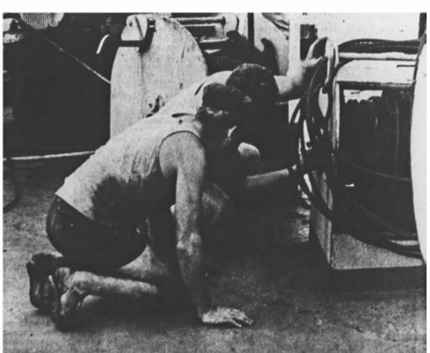
French seamen repairing a winch used to haul cargo aboard ship
